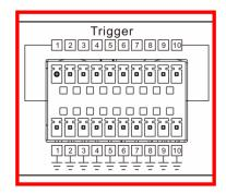
10 Inputs are provided that can be mapped to various functions of the EN12. The inputs are simple dry contact closures and are provided in ten pairs of trigger and ground connections.
